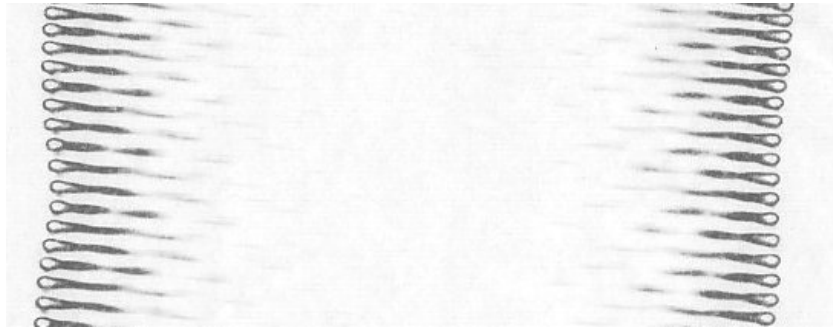
Fig. 4.9: Resonant scanner waveform on thermally sensitive paper.
