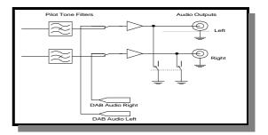
The analog stages, from the frequency to voltage demodulator, use precision, metal film, Vishay resistors. For ultimate fidelity muting is controlled by a relay which mutes the signal by shunting to 0 V to avoid relay contacts in the signal path.
