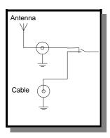
То enable FΜ stations to be received from either an external antenna or a cable feed, two antenna connections have been provided. The FΜ AGC automatically caters for the nominally higher strength
