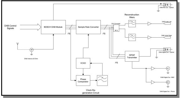
T32R DAB card schematic block diagram
